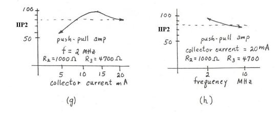
All of the graphs of Fig. 3 were developed for CBTF amps using a 1:11:4 feedback transformer, i.e., for 12 dB nominal power gain CBTF amps. Similar results may be obtained for CBTF amps with other turns ratios, but I have not made exhaustive studies of those cases, merely some spot measurements to determine if the results for those other cases were similar (they were).
