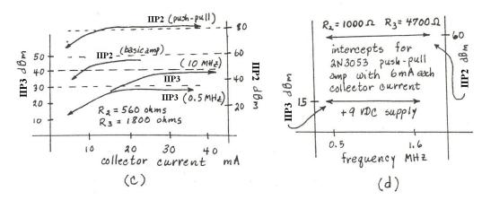
Fig. 3(c) compares the relationships between IIP (2 and 3, push-pull and basic amps) and collector current. It
