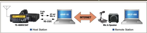
Using the ARHP-10 radio host program\*, you can even control the transceiver remotely over a LAN or via the Internet. The Kenwood Network Command System further enables VoIP (Voice over Internet Protocol) applications.
